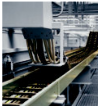
Robotics: quiet running, high acceleration, up to 10.000 cycles per day, System E4/4
