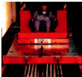
Crash test unit: 22 m/s speed and 784 m/s² acceleration, travel speed ► page 1.19
