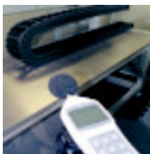
Noise level tests in igus® own acoustic laboratory
