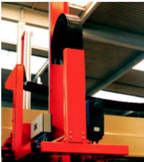
U-shaped supported e-tube for high lateral acceleration
