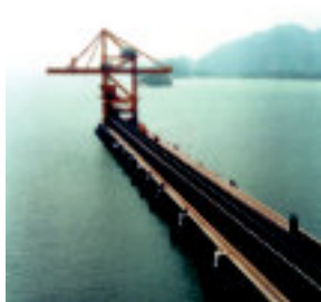
Long travels (441 m) with rol e-chain®. Long travel applications ► page 1.16
