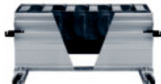
Demonstration: Guide troughs with glide bars. We recommend the use of polymer glide bars from igus® made of igulen. They are optimally matched to the e-chain® material and achieve the lowest values for friction, noise and wear.
