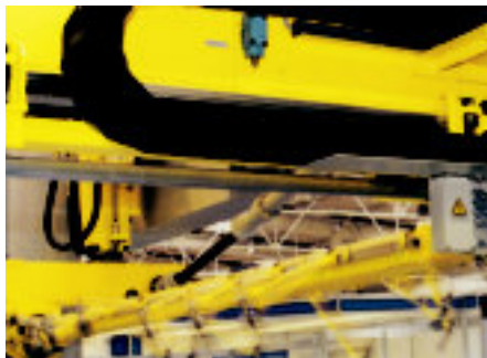
System E4 partially unsupported - please consult igus® regarding this type of configuration
