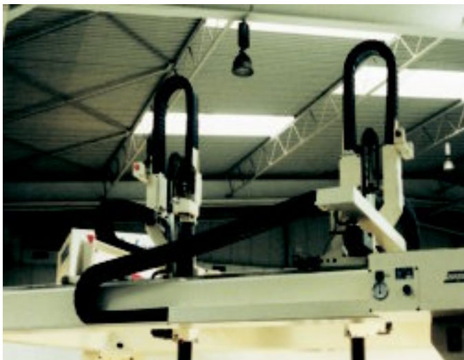
Standing application with support of the first e-chain® links - R68 e-tube
