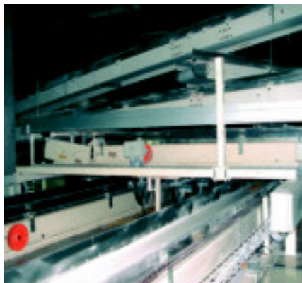
Safe energy supply also under strong dust and dirt accumulation with igus® micro flizz®
