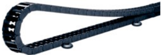
3 autoglide glider and floor guide as single parts. Glider and floor guides every 2 m completely replace a guide trough
