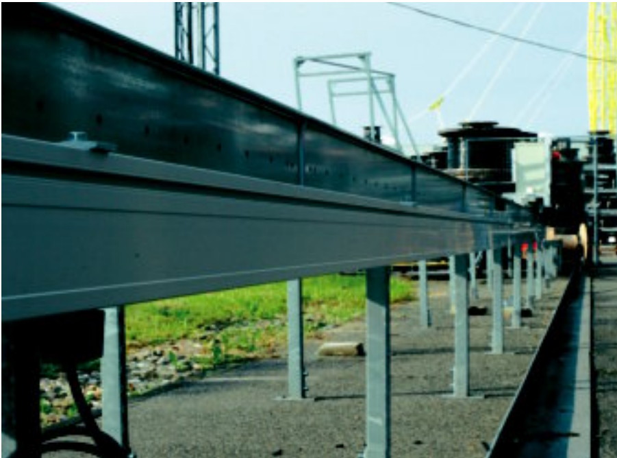
● s = 40 \text{ m} ● v = 4 \text{ m/s} ● a = 1 \text{ m/s}^2 ● m_{\text{Chain}} = 0,21 \text{ kg/m} ● m_{\text{Cable}} = 0,09 \text{ kg/m} ● Filling: 1 x CF98.05.04
