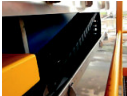
Successful application with P4.56 on a new RMG crane. 130 m travel length at 150 m/min speed. Equipped with igus® chainflex® motor-, control- and fiber optic cables
