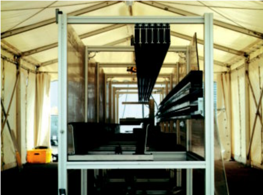
● s = 8,5 \text{ m} ● v = 4 \text{ m/s} ● a = 4 \text{ m/s}^2 ● Filling: 1x CF9.15.04 ● Running performance ca. 15.000 km without failure (issue 06.2006)
