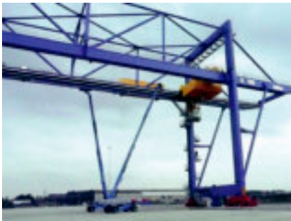
Successful application with P4.56 on a new RMG crane. 130 m travel length at 150 m/min speed. Equipped with igus® chainflex® motor-, control- and fiber optic cables
