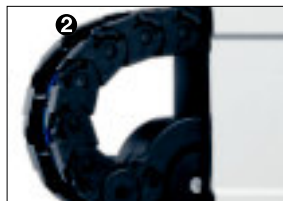
Separated upper and lower run: Running trough the radius, integrated winglets fold in
