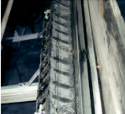
Test - Glide strips minimize wear after 1.653.187 cycles, 4.300 km
